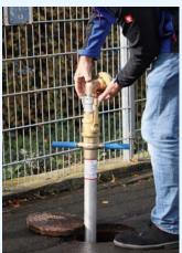
Shut off the MODU lower section and remove the MODU flushing head by opening the camlock coupling.
